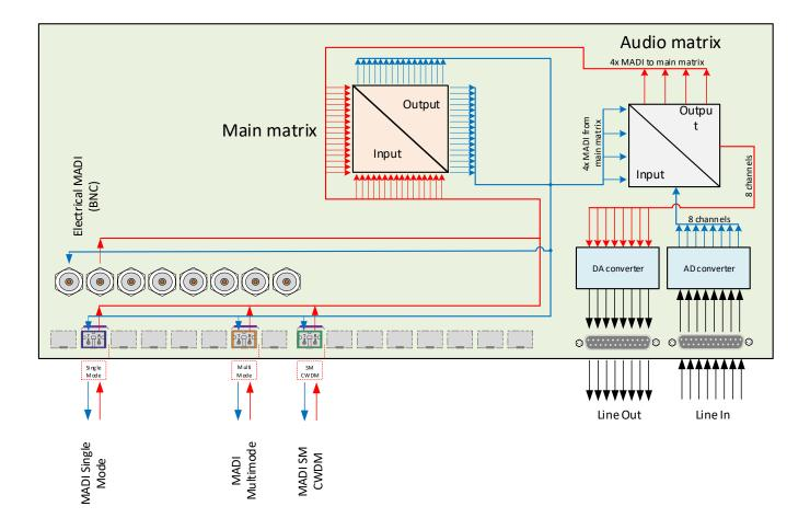
8 channels of balanced analog line level audio are converted to digital audio. Via the 264x264 audio matrix the signals can be distributed to random channels of 4 MADI streams. Input sensitivity of each analog channel is configured to +18dBu or +24dBu individually.
